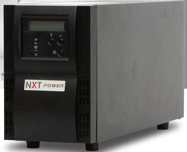
The NXT Power Vanguard Series is a double conversion topology UPS system. It provides true sinewave output to critical applications and equipment that requires seamless power correction. The VANGUARD UPS line offers generator compatibility and delivers continuous AC Power with zero transfer time. It's high frequency mode along with advanced battery management makes it eco-friendly.
