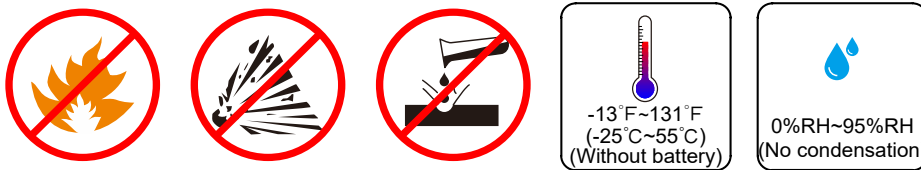
Figure1-7 Storage environment requirements
