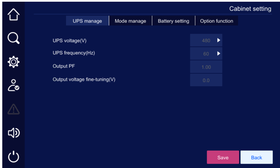
Figure5-31 Cabinet setting-UPS manage page
